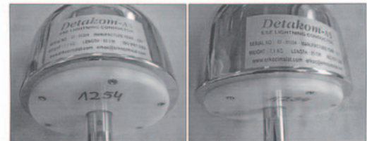
Figure 6 and 7: Test sample 1254 before and after the impulse current test
