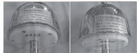
Figure 8 and 9: Test sample 1253 before and after the impulse current test
